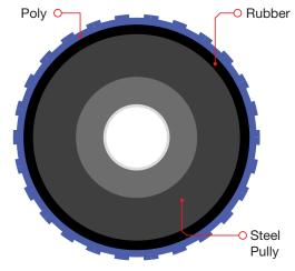
Creates robust bonding layer wear-resistant poly to pulley
