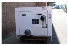
MATERIAL SUCTION INLET - 100mm male quick connect coupling.
