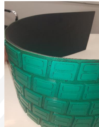
3 Rubber backed, cold-bonded, polyurethane pulley lagging
